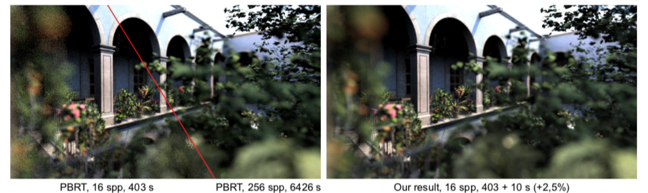
Figure 1: A scene with complex occlusion rendered with depth of field. Left: Images rendered by PBRT [Pharr and Humphreys 2010] using 16 and 256 low-discrepancy samples per pixel (spp) and traditional axis-aligned filtering. Right: Image reconstructed by our algorithm in 10 seconds from the same 16 samples per pixel. We obtain defocus quality similar to the 256 spp result in approximately 1/16th of the time.
