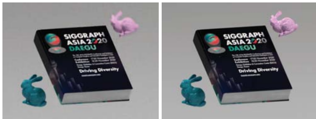
Fig. 14. Comparison of a rendered test view (left) with its reference (right) on the Book scene. The reference image has infinite depth of field. When encoding the light field onto a display of 12.5 mm thickness, only limited depth of field (left) is exhibited.
