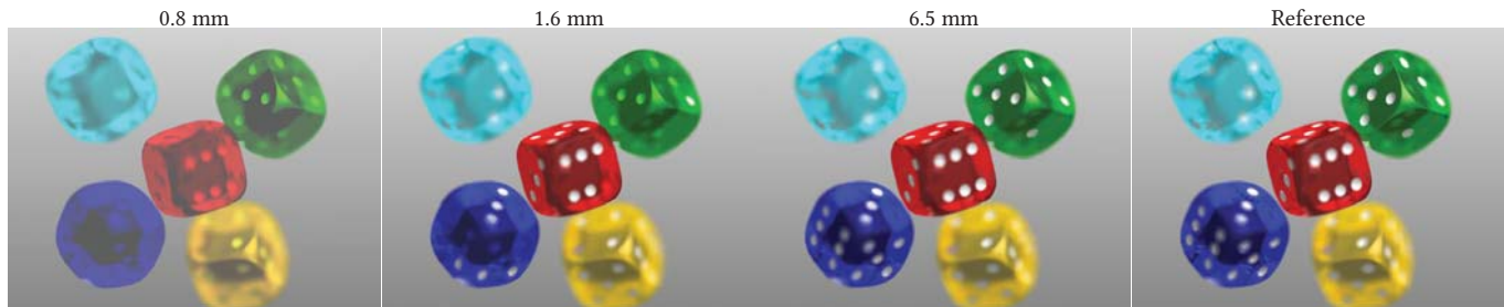
Fig. 13. Investigation of display thickness. We train neural networks to encode a light field of the Dice scene using different thickness of the display. Small thickness leads to contrast loss. Note the bright dots on blue and red dices are missing for thickness 0.8 mm and 1.6 mm.
